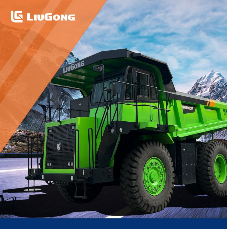
**Max. Gross Machine Weight** 88,500 kg **Net Machine Weight** 38,500 kg **Payload** 50,000 kg **Engine** HL001 500 kW (671 hp / 680 ps) @ 1,050 rpm **Rated Power Max. Speed** 55 km/h **Reverse Speed** 10 km/h **Struck Capacity** 27 m<sup>3</sup> **Heaped Capacity (SAE 2:1)** 35 m<sup>3</sup>
